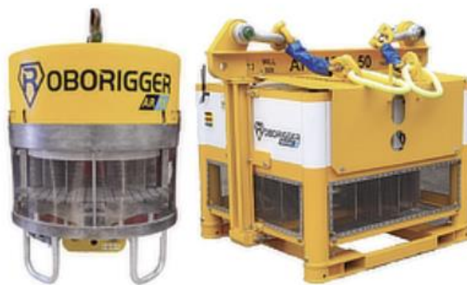
Figure 12: Roborigger has a finned flywheel which is powered by an electric motor. It attaches directly to the hook and turns the hook itself. The fins on the flywheel help to produce external thrust against the wind.
