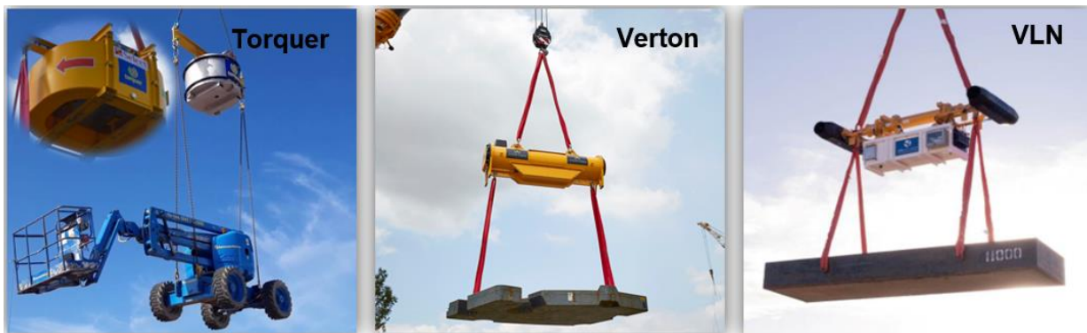
Figure 11: Torquer HALO, Verton & Vita Load Navigator devices are examples of below the hook load control devices which allow the load to be rotated. What they won't do is increase the upper limit of the crane's in service wind speed.
