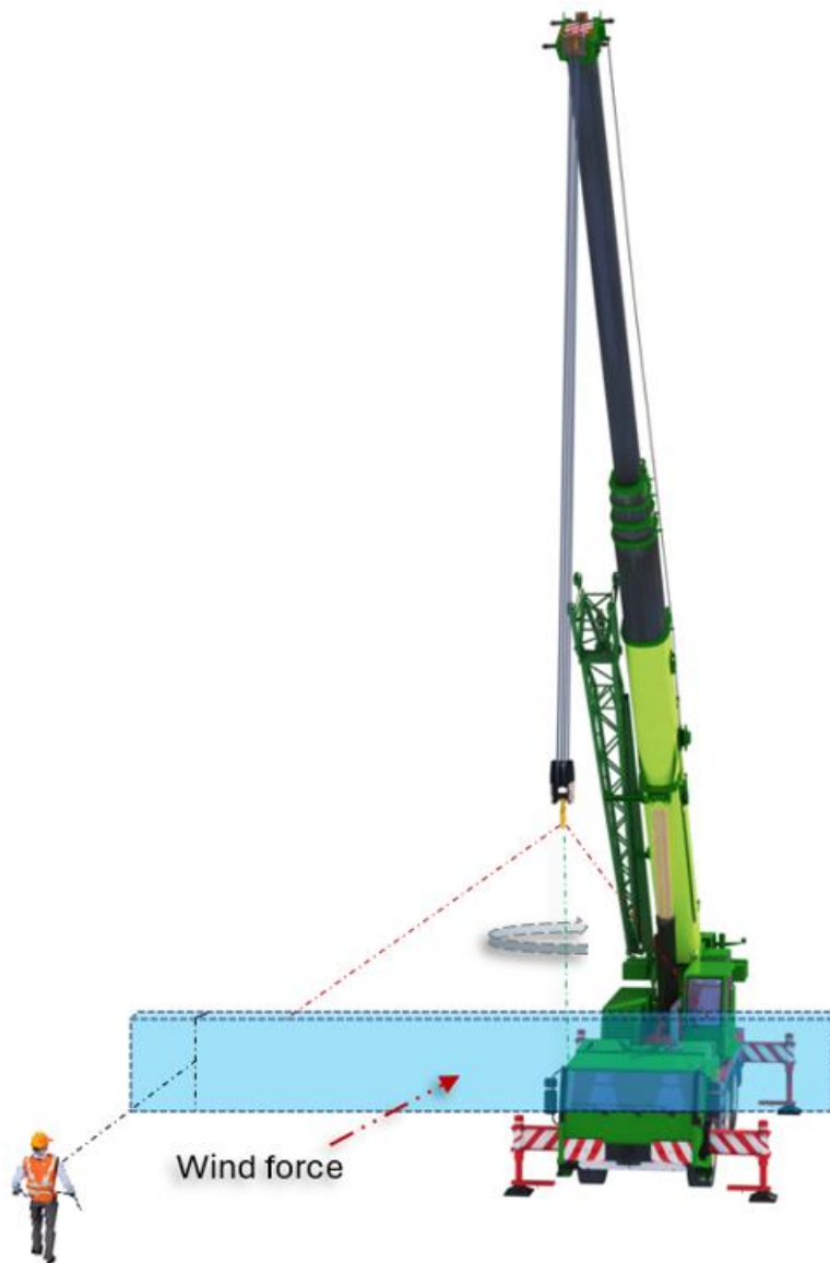
Figure 9: Image shows that because the centre of gravity of the load is not in the geometric centre of the beam, it will rotate until there is an equal projected wind area on each side of the centre of gravity, on the centre of the crane's hook.
